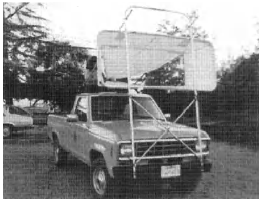
Figure 13.4. Truck-mounted trap for collection of flying insects (courtesy of Robert K. Washino).
