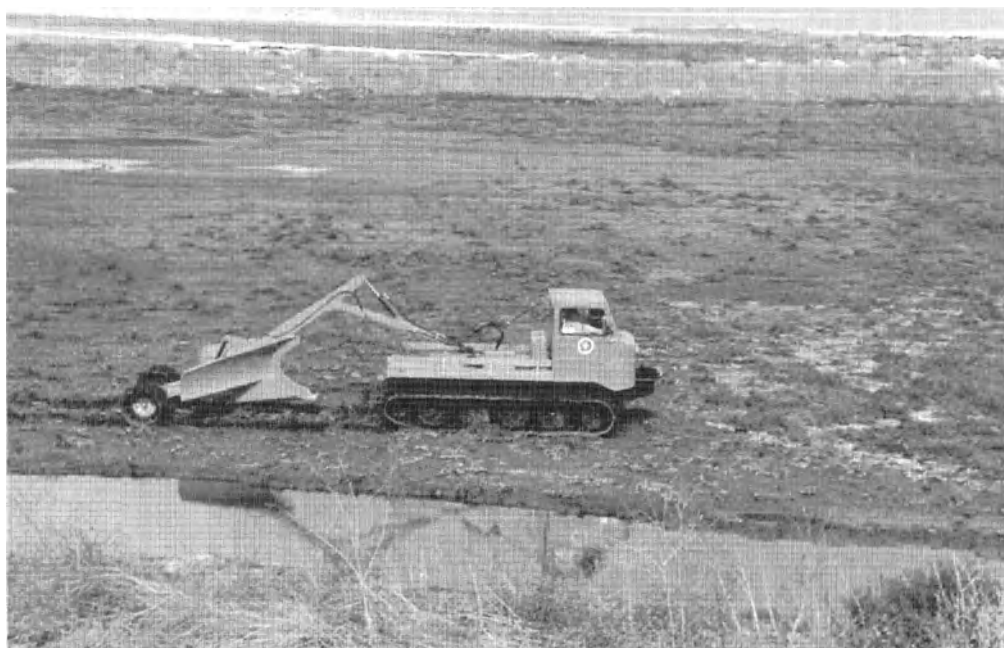
Figure 14.6. Modern marsh management for mosquito control using Thiokol® ditching equipment (photograph by John R. Rusmisl, courtesy of Alameda County Mosquito Abatement District).
